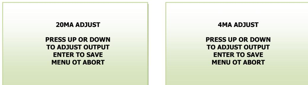
6. While measuring the output value on a meter, use the UP/DOWN keys to adjust the value up or down until the meter reads 20mA.
