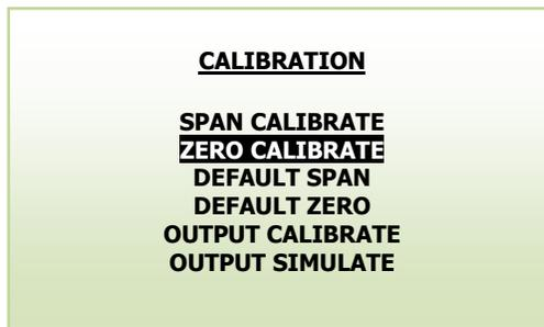
Allow the zero gas to flow through the transmitter until a stable oxygen reading is obtained. This may take from several minutes to a few hours. It is highly recommended to monitor oxygen trend on a chart recorder to ensure that the oxygen reading has stabilized; evidenced by a horizontal trend.
