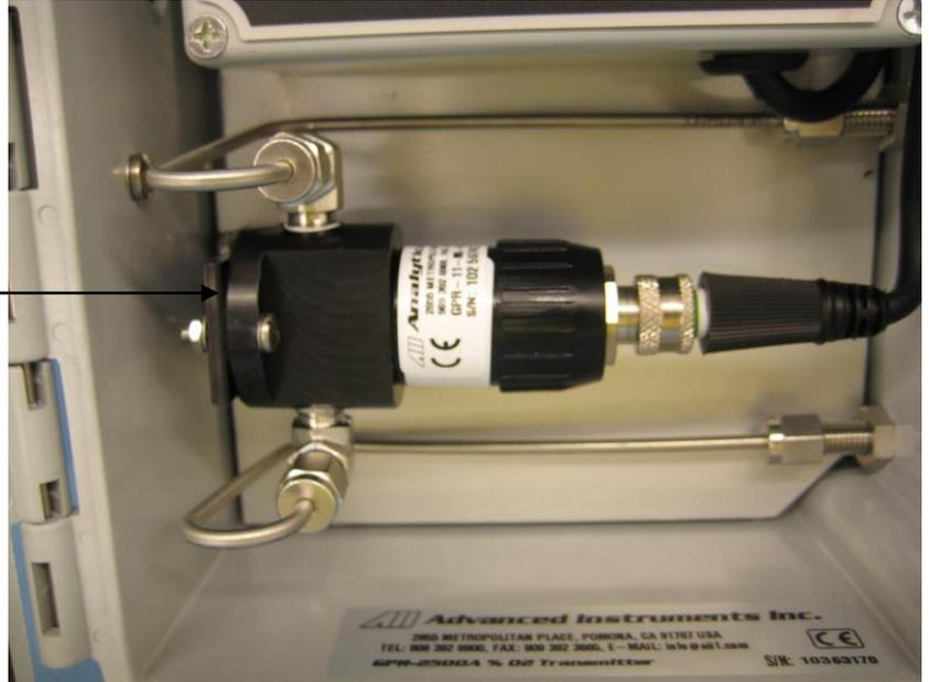
**Note:** All transmitters must be calibrated once the installation has been completed and periodically thereafter as described below. Following the initial installation and calibration, allow the transmitters to stabilize for 24 hours and perform a calibration again with a certified span gas.
