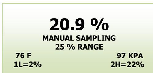
The display will not shift automatically. Instead, when the oxygen reading (actually the sensor's signal output) exceeds 110% of the upper limit of the current range an OVER RANGE warning will be displayed.
