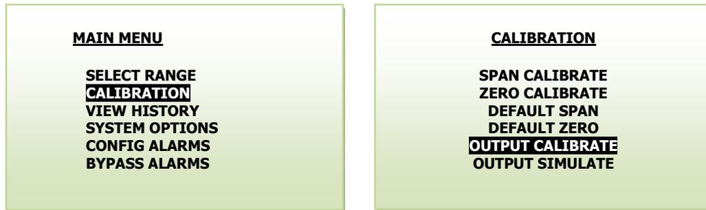
4. Advance the reverse shade cursor using the ARROW keys to highlight OUTPUT CALIBRATE.
