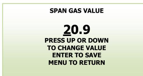
Press the ENTER key to advance the underline cursor right or press the MENU key to advance the underline cursor left.
