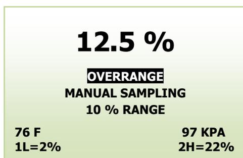
Once the OVER RANGE warning appears the user must advance the transmitter to the next higher range via the menu and keypad Press MENU, select MANUAL SAMPLING, press ENTER, select the appropriate MANUAL RANGE and press ENTER again.
