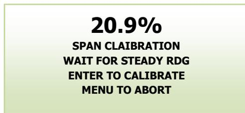
Allow approximately 5-10 min for oxygen to stabilize and then press ENTER to complete span gas calibration
