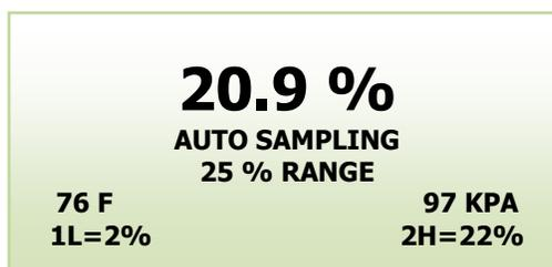
The display will shift to the next higher range when the oxygen reading (actually the sensor's signal output) exceeds 99.9% of the upper limit of the current range. The display will shift to the next lower range when the oxygen reading drops to 85% of the upper limit of the next lower range.
