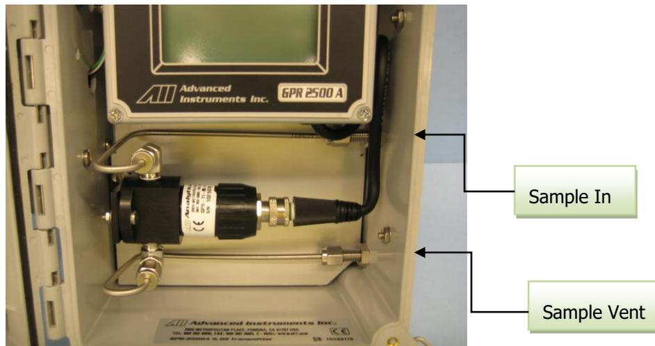
Flow rates of 1-5 SCFH cause no appreciable change in the oxygen reading. However, flow rates above 5 SCFH generate backpressure and erroneous oxygen readings because the diameter of the integral tubing cannot evacuate the sample gas at the higher flow rate. A flow indicator with an integral metering valve upstream of the sensor is recommended as a means of controlling the flow rate of the sample gas. A flow rate of 1-2 SCFH or 0.4-1 liter per minute is recommended for optimum performance.
