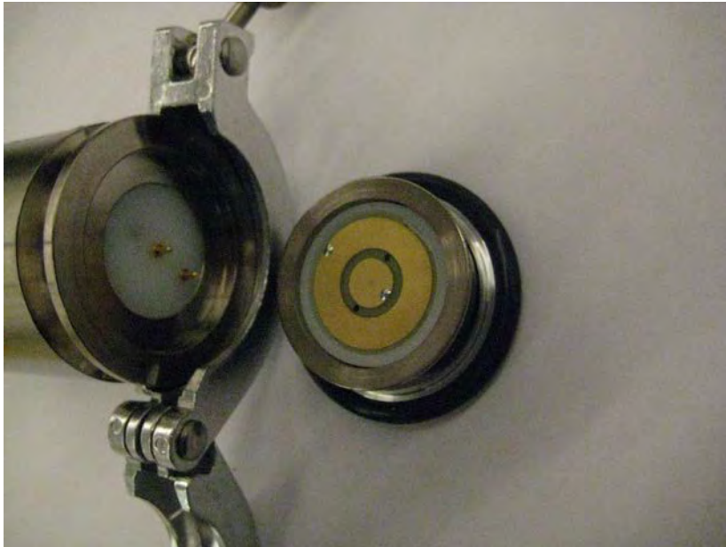
Upper section, the clamp, sensor holder and flange o-ring
