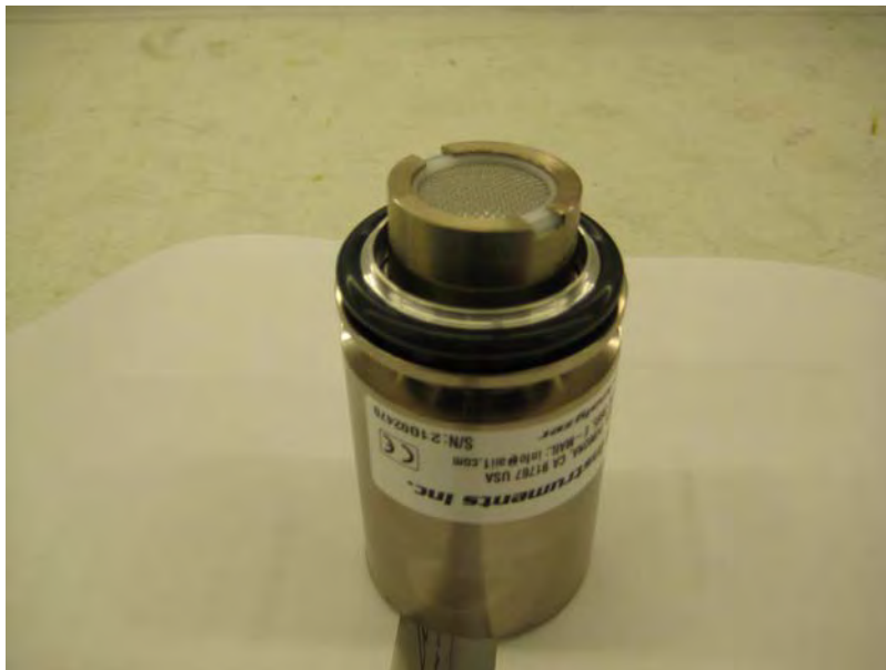
Upper section with sensor holder containing sensor and the flange o-ring ready to be installed on the flange of a pipe
