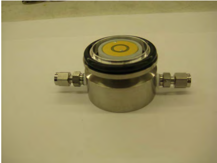
Optional flow through KF-40 flange shown with sensor
