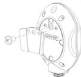
A-3657 Dovetail Bracket HRWR-1162 Screw 1/4-20 x 3/8"
